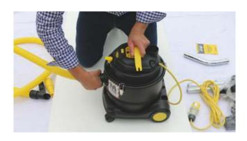
14 Turn clockwise to lock (gently pull to ensure it is locked)
