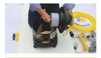
1 Ensure the filter retainer screw is tight
