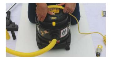
Plug in device then press switch to turn extraction on/off
