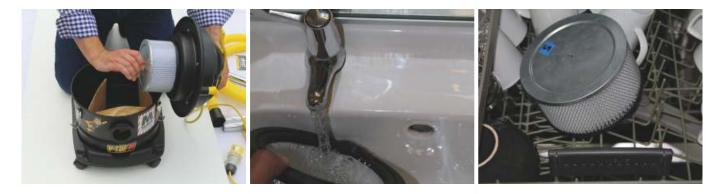
22 If red monitor continues the filter may need washing. Undo filter retainer screw, remove filter and wash with warm soap water (this can by done by hand or in dishwasher). Filter must be allowed to dry thoroughly before refitting.
