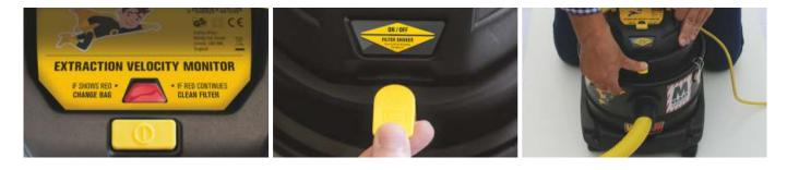
If monitor is red, press and hold Filter Shaker button for 10 seconds to clear filter (device/extraction must be on) If the monitor turns red only as and when you connect it to your power tool, ensure that the extraction passages of your tool are not blocked. If clear, it is OK to use. Just check the flow periodically by removing the extraction hose.
