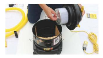
24 Refit filter and retainer screw and tighten
