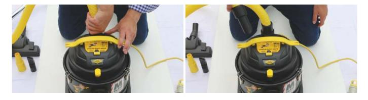
To use the blow feature, simply connect the hose to the exhaust port on top of the unit (as you would to the suction port)
